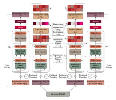
The transformer-based architecture used in FragNet
